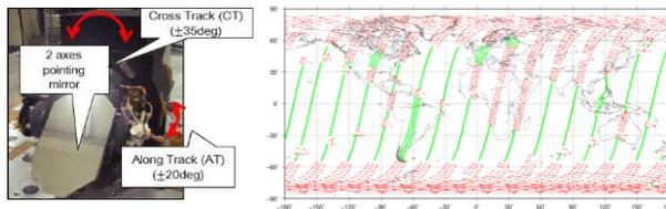
Targeting CH<sub>4</sub> large emission source and mega cities with an agile pointing system by uploading the pointing-angle table every day.
